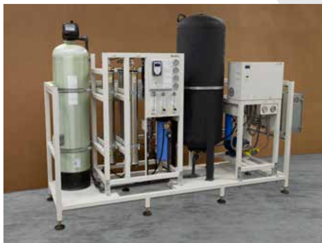
Custom rack systems Single-point water, steam, drain, and power connections
