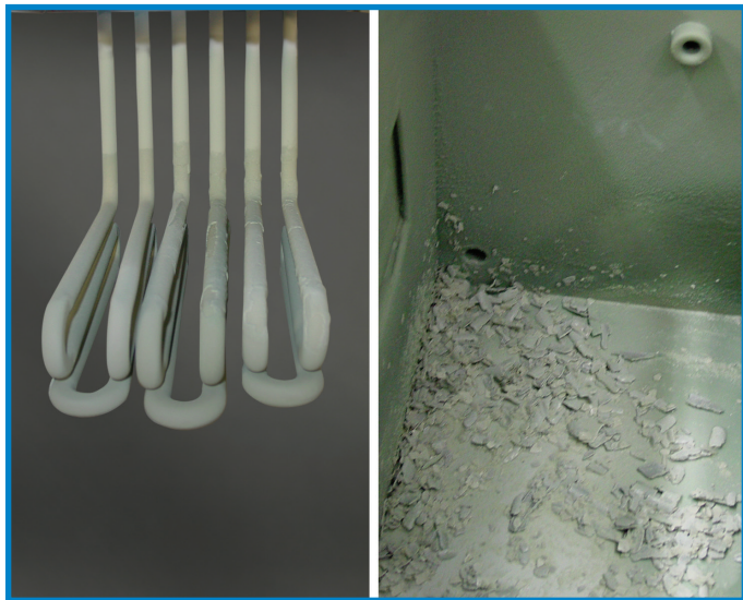
Untreated supply water causes scale buildup
