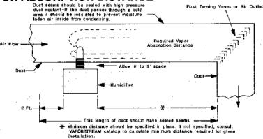
A distance of air travel is required for the steam to "disappear" or go into the gaseous state.
