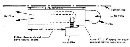
In an application where no duct system exists, or if the duct air is too cool for proper humidity absorption, a recirculation fan can be used. The fan circulates room temperature air across the LTS humidifier and discharges humidified air into the space. The point of discharge should be carefully selected to avoid condensation on surfaces of the building or equipment.
