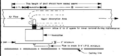
Minimum distance should be specified in plans. If not specified, consult VAPORSTREAM catalog to calculate minimum distance required for given installation.
