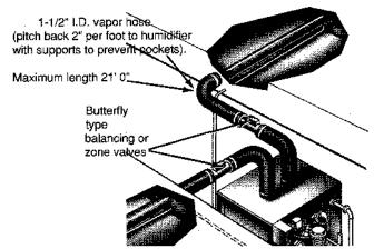
Humidifier should be mounted level - both directions.
