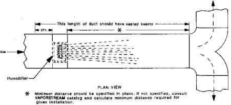
When a LTS humidifier is installed upstream of a duct split, the humidifier should span most of the duct width or be centered upon it to equalize the humidifying effect between the two branches.
