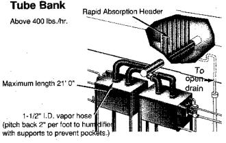
Humidifiers should be mounted level - both directions.
