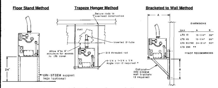
\*Due to the size and weight of the LTS 200, the trapeze hanger method is not recommended.
