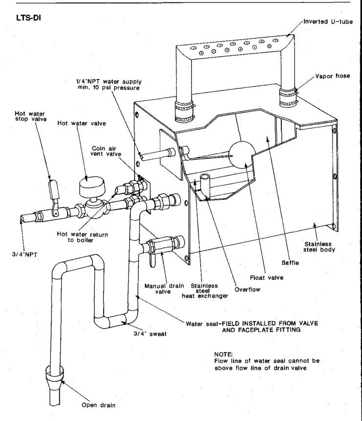
NOTE: Drain piping material must be suitable to handle 212° F (100°C) water.
