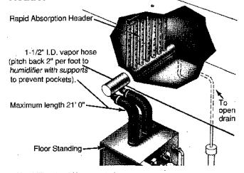
Humidifier should be mounted level - both directions.
