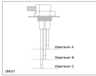
A conductivity probe system allows VAPOR-LOGIC<sub>2</sub> to control water levels for optimum operating efficiency. The three-probe system is monitored by the VAPOR-LOGIC<sub>2</sub> control, which performs all the necessary logic and timing functions to provide total water level control and safety shutdown.
