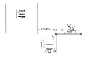
**Figure 4-4:** The STS and LTS humidifiers offer the flexibility of mounting the VAPOR-LOGIC<sub>2</sub> key pad on a control cabinet that is mounted on either the humidifier or on a wall near the humidifier.
