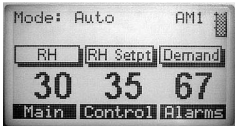
This is the Idle Screen displayed with Vapor-logic3 versions 5.x.x (systems with multi-tank configuration capability)
