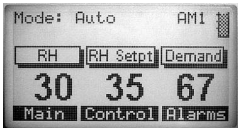
This is the Idle Screen displayed with Vapor-logics versions 5.x.x (systems with multi-tank configuration capability)
