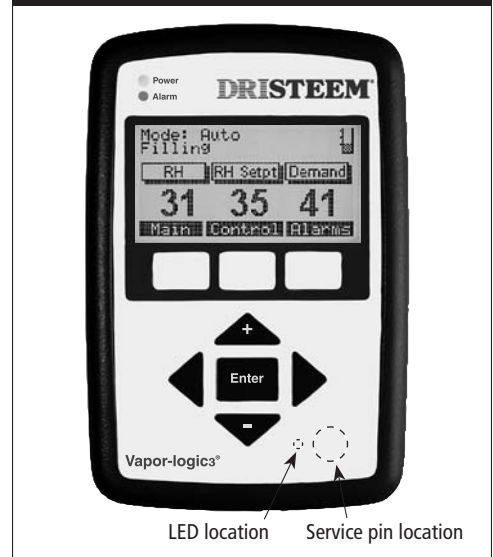
Figure 37-1: Display service pin and LED locations
