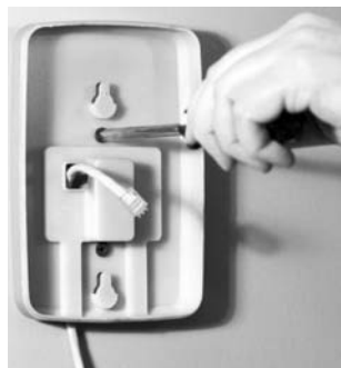
Figure 17-2: Mounting the keypad/display
