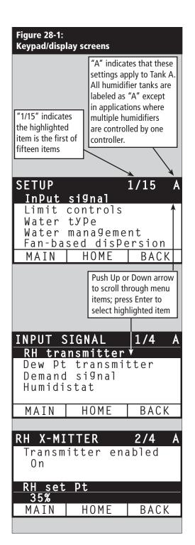
To simplify the field-installation process, humidifiers are sent from the factory configured as ordered. However, some settings are unknown at the factory and need to be defined during the setup process using the Setup menu. The Setup menu is also where you make future system setting changes.
