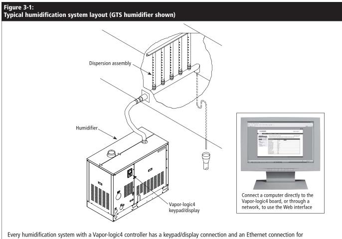
connection to a Web interface on a computer. A GTS humidifier is shown here, with keypad/display mounted on the cabinet. Other types of DRI-STEEM humidifiers can have the keypad/display contained within a control cabinet or mounted remotely.
