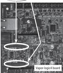
3. Connect wiring from LonTalk system to LON ProtoCessor module on
