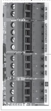
Field connection terminals have labels printed on a white border.
