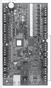
Terminals P-11 through P-16 have a white border on the Vapor-logic4 board. This is where you will make most of your field wiring connections.
