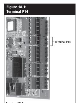
Terminal P14: 24vdc = Power to auxiliary temperature sensor or temperature compensation sensor (transmitter) TS = Auxiliary temperature sensor or temperature compensation sensor (transmitter) (4-20 mA input)
