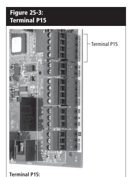
24vac = Power to combustion air switch CAsw = Combust. air sw. (24vac input) 24vac = Power to power vent switch PVsw = Power vent switch (24vac input)
