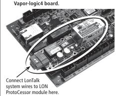
**NOTE:** Orient the LON ProtoCessor module as shown, with wire connectors end at the side of the Vapor-logic 4 board.
