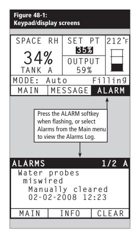
The Alarms menu displays system alarms. Using the keypad/display, go to the Alarms menu by pressing the Alarms softkey (which will be flashing if there is an Alarm), or by pressing the Home softkey and then the Alarms softkey. Using the Web interface, click on the View Alarms link in the upper left corner of any screen.
