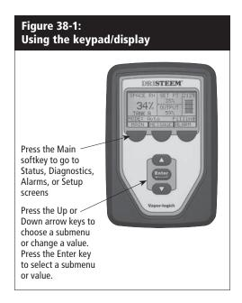
Vapor-logic4 keypad/display has the following menus and screens:
