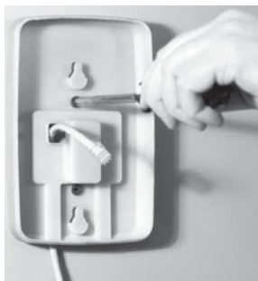
Figure 19-2: Mounting the keypad/display
