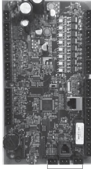
Terminals P-11 through P-16 have a white border on the Vapor-logic board. This is where you will make most of your field wiring connections.
