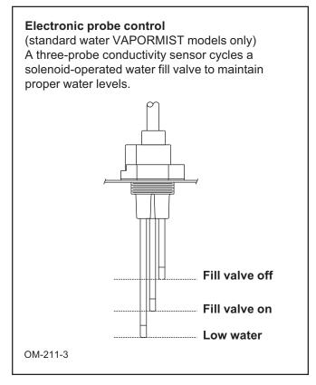
VAPOR-LOGIC<sup>®</sup> control VAPOR-LOGIC<sub>3</sub> is the standard controller for the VAPORMIST. For more information regarding the operation of the VAPOR-LOGIC3 microprocessor, see the VAPOR-LOGIC, Installation, Operation and Maintenance Manual.
