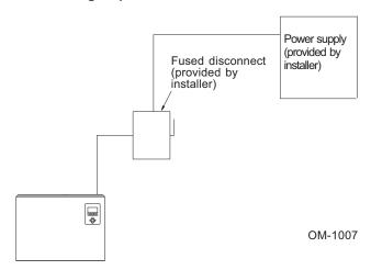
**Note:** Control wiring and power wiring must be run in dedicated or separate earthed metal conduit, cable trays or trunking.
