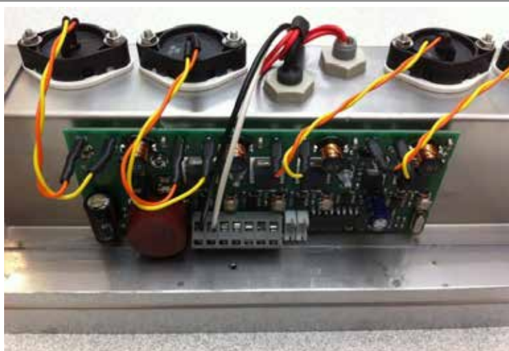
FIGURE 57-2: CORRECT WIRE ASSEMBLY (MODEL BR)
