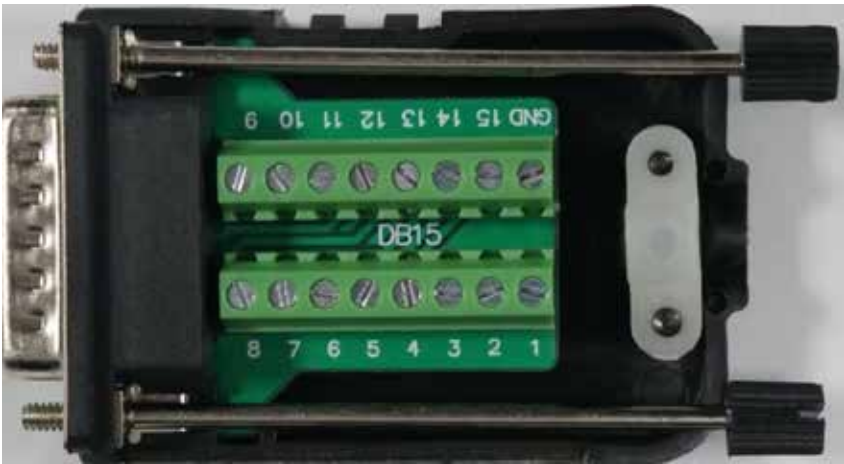
FIGURE 28-1: 15-PIN D-SUB CONNECTOR MUST BE USED FOR THE CONTROL SIGNALS FOR OPERATING THE HUMIDIFIER. EXTERNAL CONNECTION X02.
