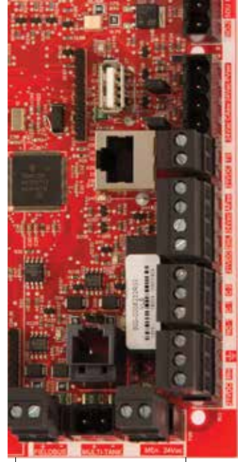
FIGURE 8-1: VAPOR-LOGIC CONTROL BOARD DETAIL
