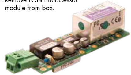
FIGURE 74-1: LON PROTOCESSOR MODULE INSTALLATION
