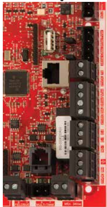
FIGURE 8-1: VAPOR-LOGIC CONTROL BOARD DETAIL
