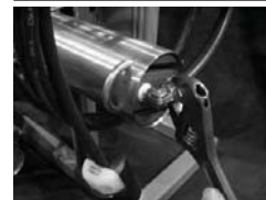
FIGURE 15-1: DRISTEEM REVERSE OSMOSIS MEMBRANES
