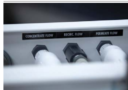
FIGURE 5-2: RECIRC FLOW LINE
