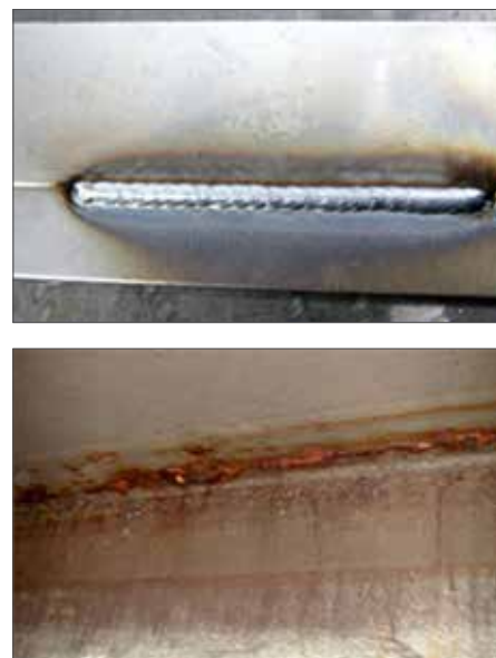
FIGURE 22-1: STAINLESS STEEL CORROSION EXAMPLES
