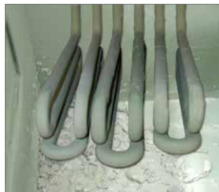
FIGURE 38-1: HARD WATER SCALE ON HEATERS AND TANK
