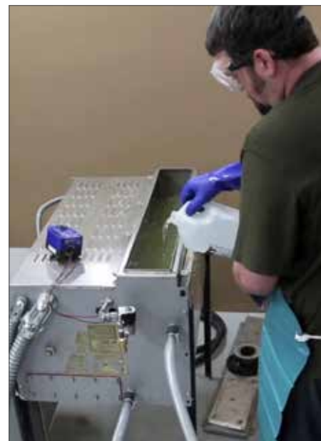
FIGURE 9-2: POURING DE-SCALING SOLUTION INTO A HUMIDIFIER TANK
