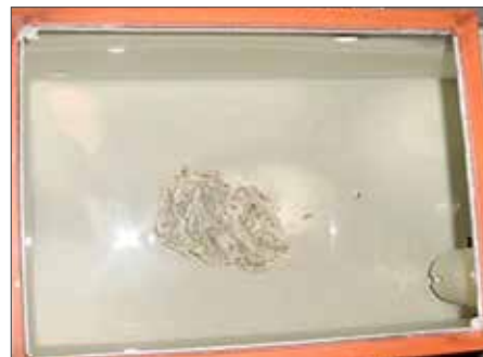
FIGURE 38-2: SOFTENED WATER RESIDUE IN HUMIDIFIER TANK
