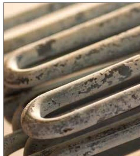
FIGURE 9-1: HARD WATER SCALE ON HEATING ELEMENTS
