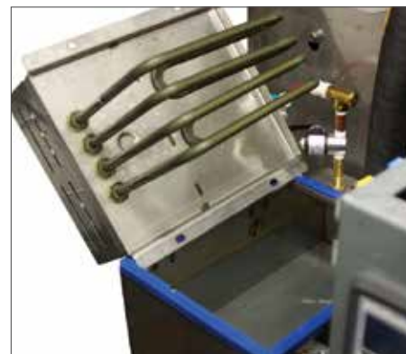
FIGURE 39-1: RO WATER LEAVES NO RESIDUE ON HEATERS AND TANK
