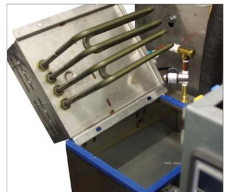
FIGURE 20-3: RO WATER LEAVES NO RESIDUE ON HEATERS AND TANK
