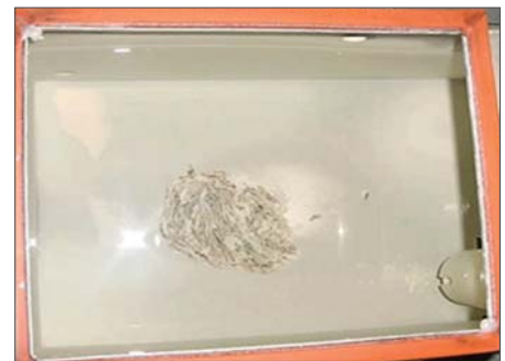
FIGURE 20-3: RO WATER LEAVES NO RESIDUE ON HEATERS AND TANK
