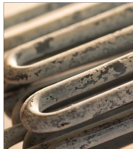
FIGURE 9-1: HARD WATER SCALE ON HEATING ELEMENTS
